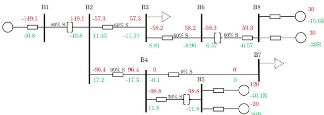
Fig. 2. High generation initial dispatch: active and reactive power flows
