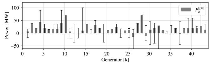
Fig. 4. HV distribution grid: Initial active power schedule and power limits
